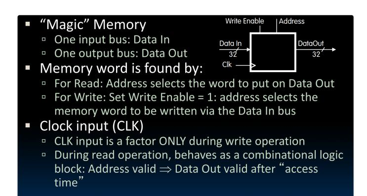
For **read** operation we **don't** need to wait for the clock, just put the address of register or memory, the data will automatically pop up.
