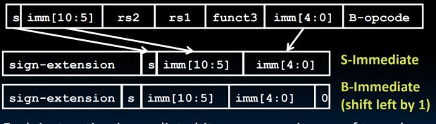
Each instruction immediate bit can appear in one of two places in output immediate value – so need one 2-way mux per bit
