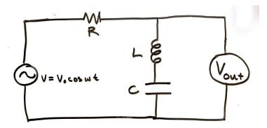
$$\tilde{I}_0(t) = \frac{V_0}{R + i\left(\omega L - \frac{1}{\omega C}\right)} \tag{38}$$
