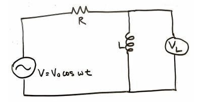
If this were a resistor, we would use Ohm's law (V = IR) to find the voltage drop across the resistor since we now know the current through it. The equivalent statement using impedances is
