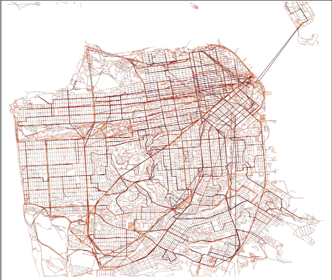
Figure A2-1. Integrated high-frequency microtransit, public transit and pedestrian network by travel time during the morning peak period in San Francisco.
