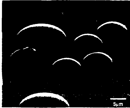
Figure 3.6: After the annealing process, round photoresists become dome-shaped.
