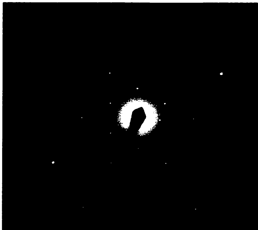
Figure 5.4: Electron diffraction pattern of a C_{36} crystallite. The pattern is hexagonal with a calculated d-spacing of 6.68 Å. (Adapted from Ref. [46])
