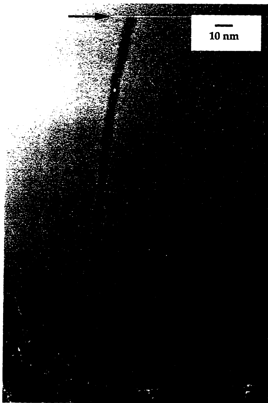
Figure 9.1: Vibrating BN nanotube at T=300\text{K} .
