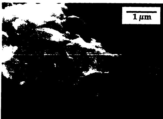
Figure 10.3: SEM image of boule sample from a combined boron, carbon and nitrogen experiment.
