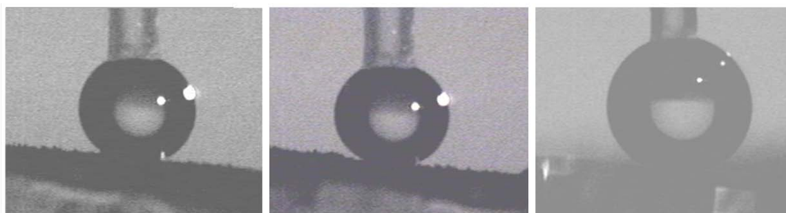
Figure 3-4. Characteristic contact angle images for VANT-PDMS composites. Droplets quickly roll off the substrate if not held by the needle. Contact angles are consistently >155^\circ . Droplets bounce off the surface when dropped from a distance. Pinning only occurs at defect sites.
