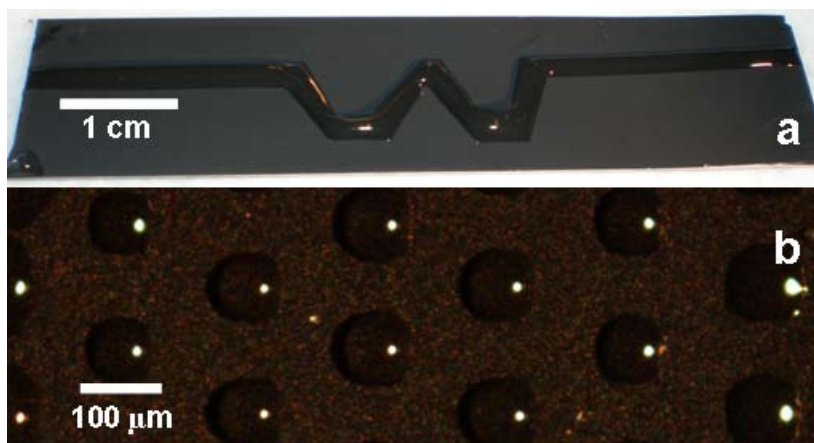
Figure 2-12. Superhydrophilic patterns on superhydrophobic backgrounds: (a) a macroscopic superhydrophilic channel; (b) dark field image of selective condensation on micro-patterned hydrophilic regions.
