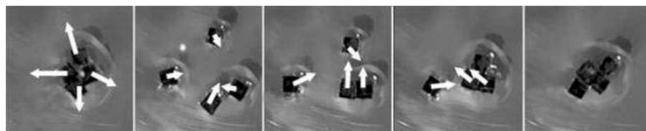
Figure 3-13. Timeline showing a light disrupted system. Mesoscale assembly of four VANT-PDMS objects (each 1 mm x 1 mm). Top view time sequence of laser induced disruption from one state (left-most panel, similar to the state of Figure 3-12b) to the reassembly to another state (right-most panel, similar to the state of Figure 3-12f). Laser irradiation only occurs at the junction between the four blocks in the first frame. Subsequent frames show capillary induced relaxation. Entire process occurs over a period of approximately three seconds. Arrows indicate instantaneous velocities. Where necessary, glare has been digitally removed for clarity.
