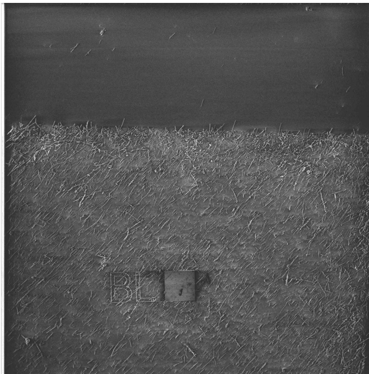
Figure 3.9: Deposition of aligned MWCNT in a functionalized area. The nanotubes were deposited in higher concentrations at the top and upper right corner as these were the first areas encountered by nanotubes flowing in solution. The alignment of spin coated nanotubes is also visible in this figure. The patterned square to the right of the letters “BL” is 10\ \mu\text{m} wide.
