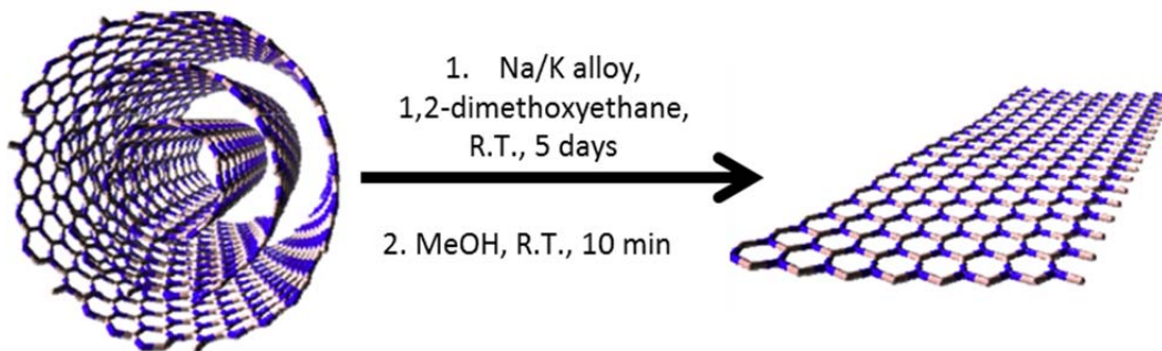
Figure 3-8 TEM micrograph of a BNNR formed through the alkali solubilized method for BNNT splitting, being pictorially represented in the lower schematic, where precursor BNNTs (left) are reacted with a Na/K alloy dissolved in dry 1,2-dimethoxyethane to form BNNRs (right) following a quench step in methanol.
