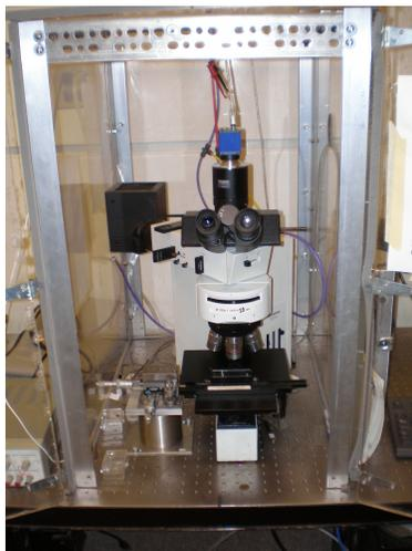
Figure 3.2: Olympus BX-50 optical microscope, Zettl group.
