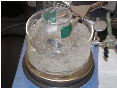
Figure 2.6: Photograph of Piranha etch of silicon wafer.
