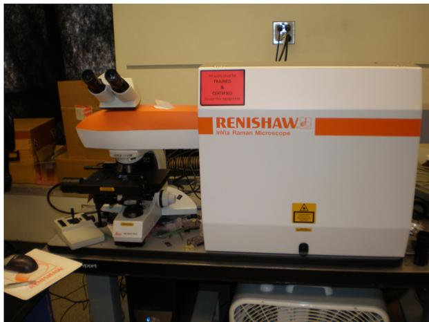
Figure 3.12: Zettl group micro-Raman spectrometer. Zettl group Wiki.
