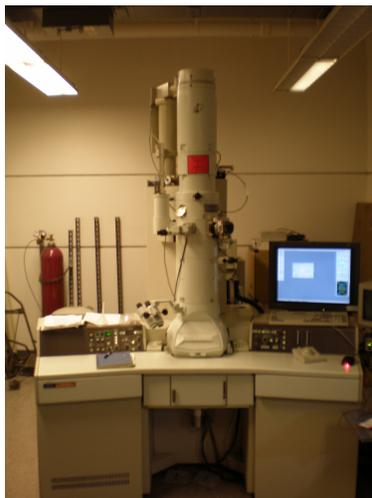
Figure 3.26: Zettl group JEOL 2100 transmission electron microscope.
