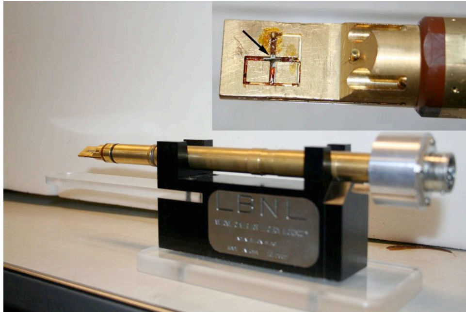
Figure 3.1: The In Situ Biasing Stage for the TEM
