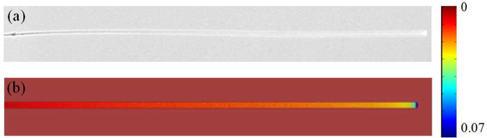
Figure 3.9: Nanotube during field emission. (a) TEM (b) FEA of 1\mu\text{m} tube located d_0 = 1\mu\text{m} from a counter electrode held at 100 V. Scale bar for surface charge density is in C/m^2 .
