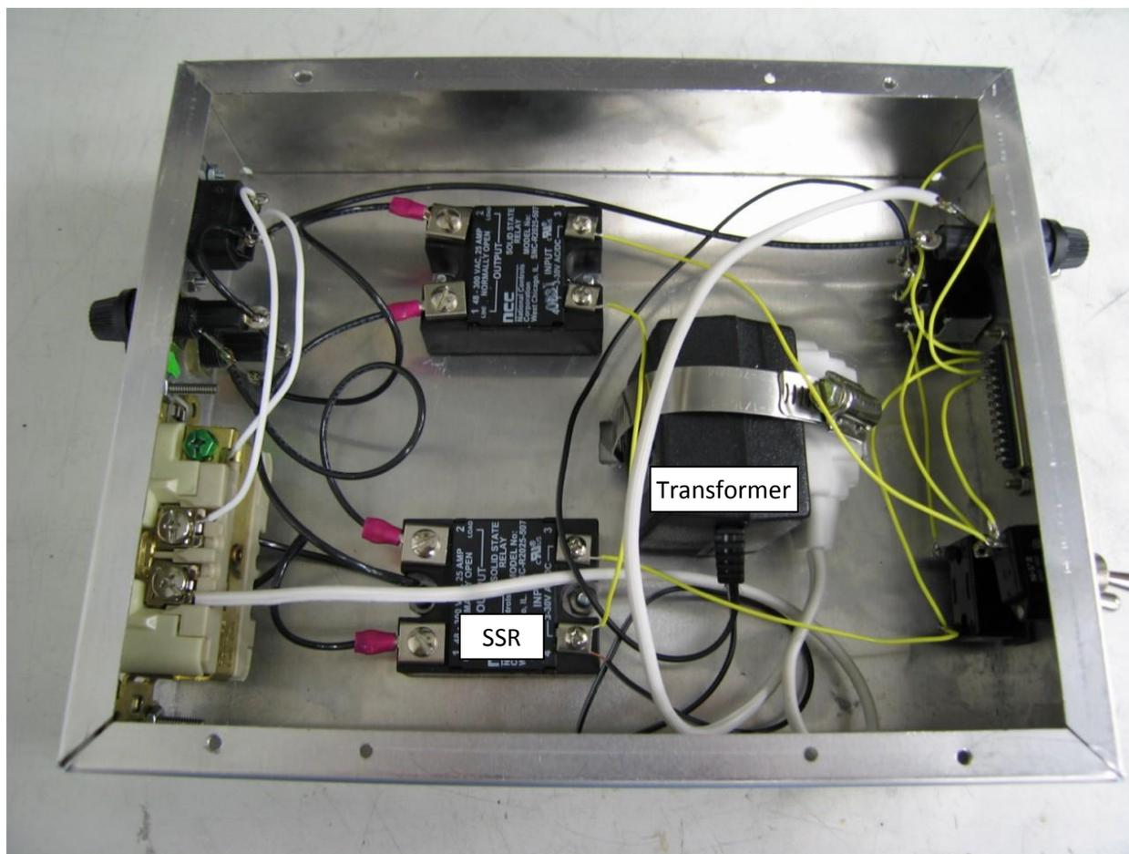
Figure 3: The inside of the fail-safe box. The solid state relays (SSR) are displayed, along with the transformer.
