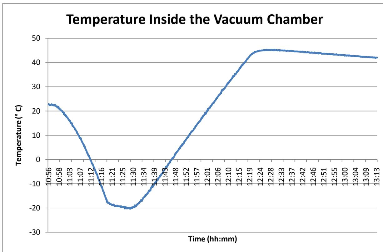
Figure 9: Temperature inside the vacuum chamber as a function of time.
