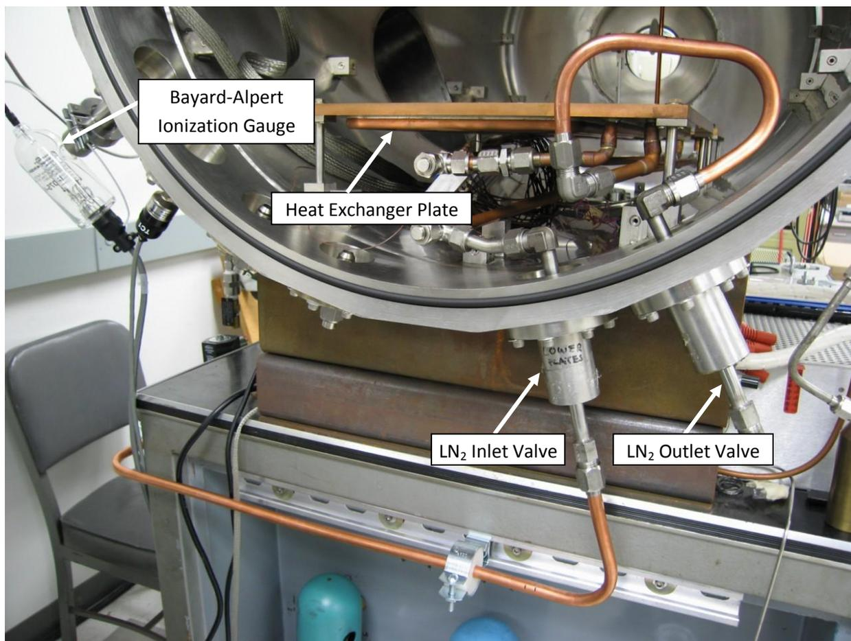
Figure 6: The inside of the chamber is visible, showing where the pipe connects to the heat exchanger. This photograph was taken before the LN<sub>2</sub> outlet piping and insulation was installed.
