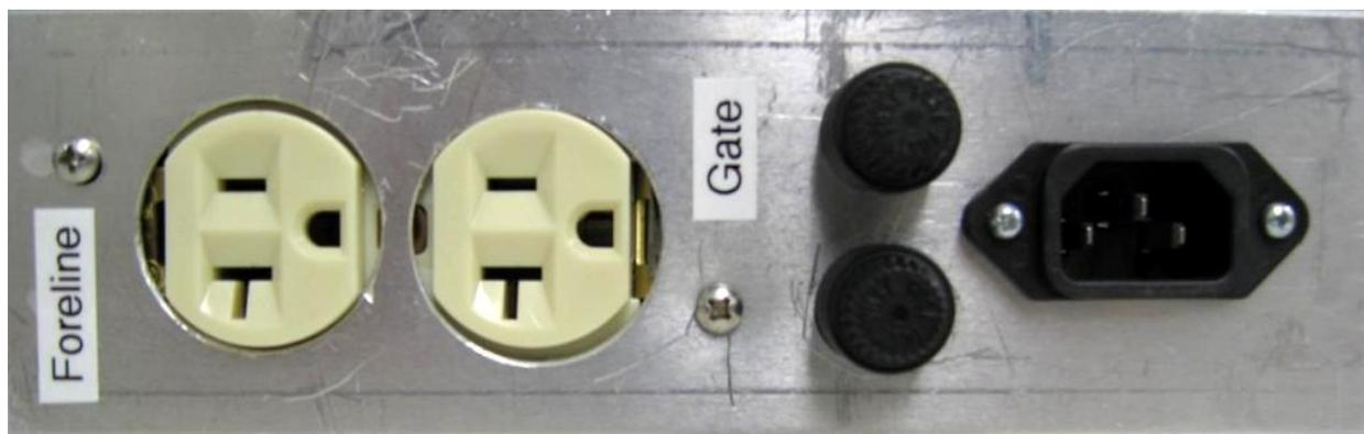
Figure 5: The back view of the fail-safe box. The electrical sockets are properly labeled to correspond to either the foreline valve or the gate valve.
