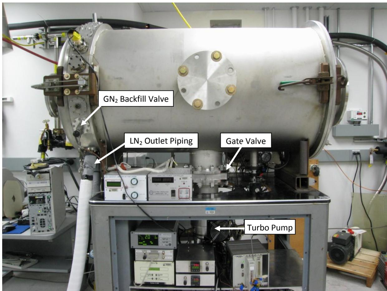
Figure 1: Photograph of the test chamber with parts labeled.
