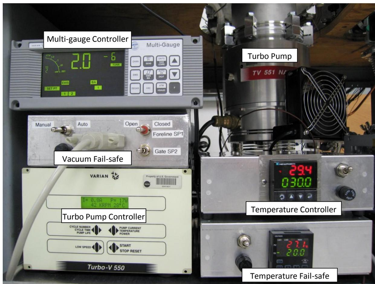
Figure 8: The controller and fail-safe setup.
