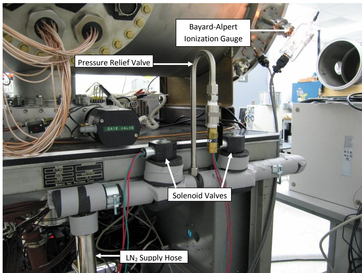
Figure 7: A Unistrut channel was mounted behind the vacuum chamber to mount the solenoid valves.
