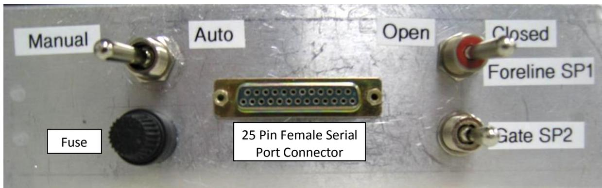
Figure 4: The front view of the vacuum fail-safe box. The left switch controls whether the unit is in manual mode or automatic mode. The switches on the right are labeled with the correct valve that the switch controls and its corresponding setpoint number when using the multi-gauge controller.
