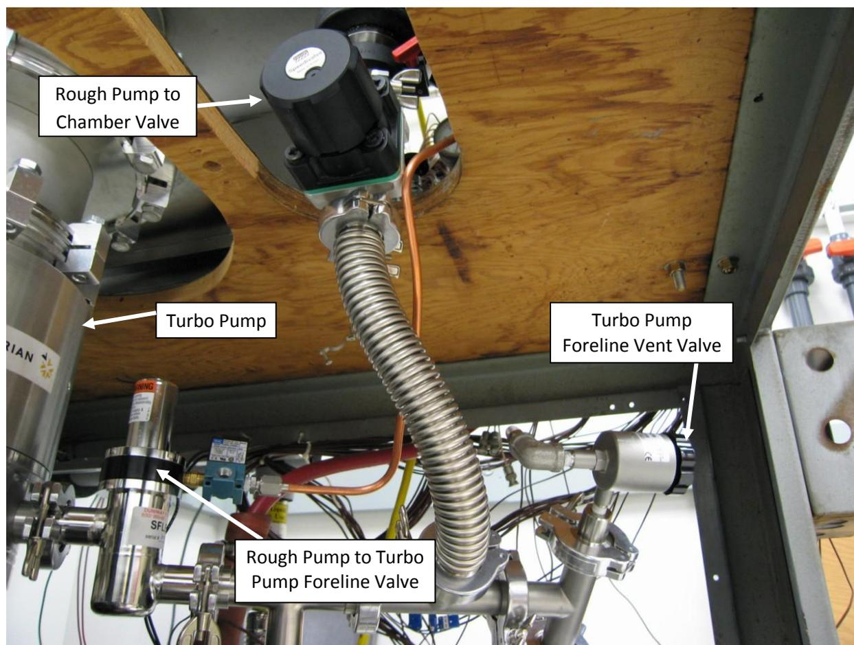
Figure 2: Detail on the valves and the turbo pump.
