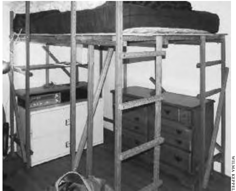
3.3b: Version 2: Better, but the file cabinet drawers bumped the dresser. Wilma put the 5 x 7 foot deck 5 feet above the floor so she could sit up in bed under the 8-foot ceiling.
