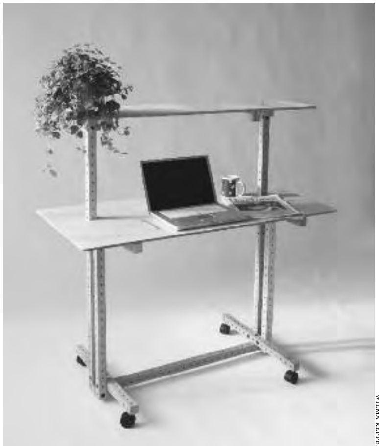
5.1: Double posts keep this "stem frame" desk square. Panels are apple plywood, with a 2 x 4 foot desk surface 30 inches high.
