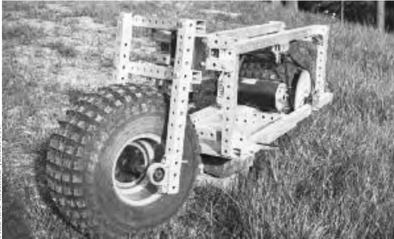
21.7a: An early version of Phil's Electric Tote Goat mounted the front axle on pillow blocks bolted to grid beam forks.
