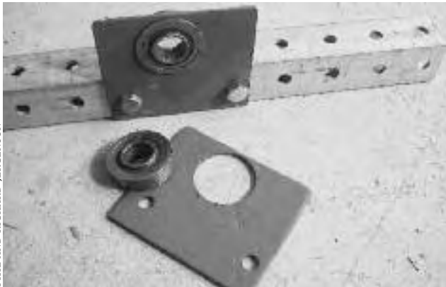
21.7b: Simple adapter plates hold flanged bearings for a Yard Truck axle. Shaft clamps on the axle hold the bearings in place. Avoid the type with a set screw. Instead, use the type that looks like a round pinch block.
