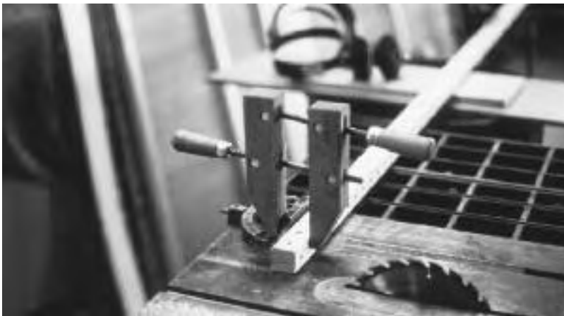
14.3: To get straight cuts on a table saw, clamp long sticks to the miter guide. The hand screw shown here won’t mar your sticks.
