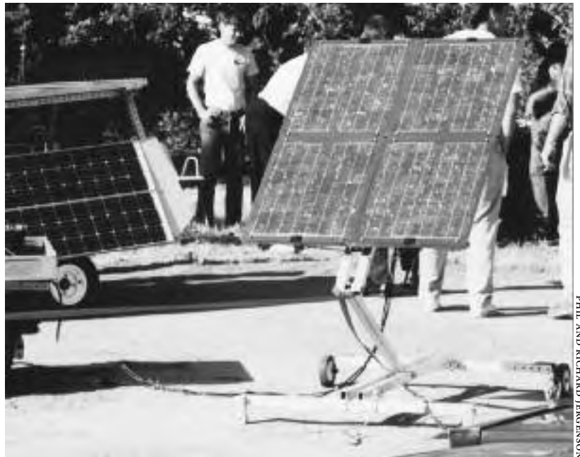
9.11: Aluminum portable tracker by George Buono.
