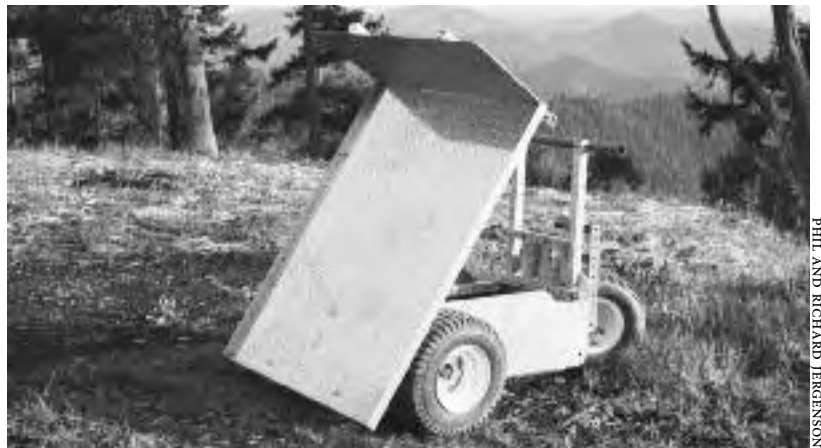
10.4: Early Yard Truck with crossbar handle and rear caster. The dump bed is aluminum diamond plate.
