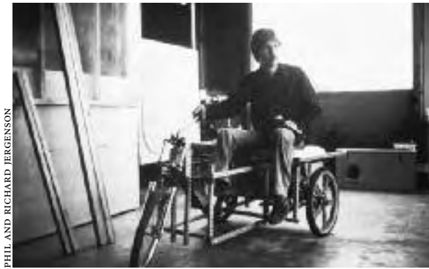
2.7: Phil's 1978 Electric Vehicle Test Bed was the first grid beam vehicle we know of. It was also the first project built using sticks with the hole pattern we use today. "Building with double-hole sticks convinced me of the advantages of pre-drilling every hole so we could put a tri-joint anywhere," Phil remembers.
