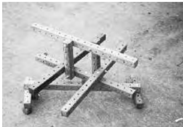
13.2: Cable turntable by Tom Blinks unrolls wire, cable or hose without twists or damaging kinks.
