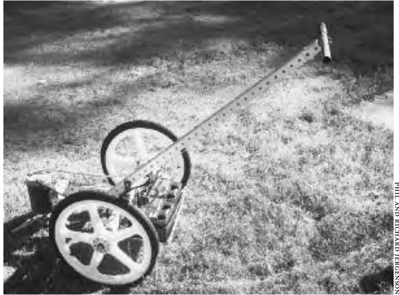
10.3: Phil's Electric Mower has a frame of 1½-inch aluminum.
