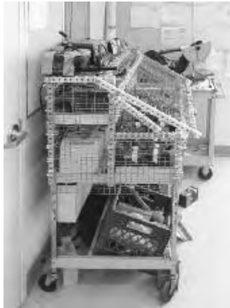
14.5: Electric Moose Club battery safe with welded wire mesh panels. Plastic wire ties attach them to the 1-inch frame.
