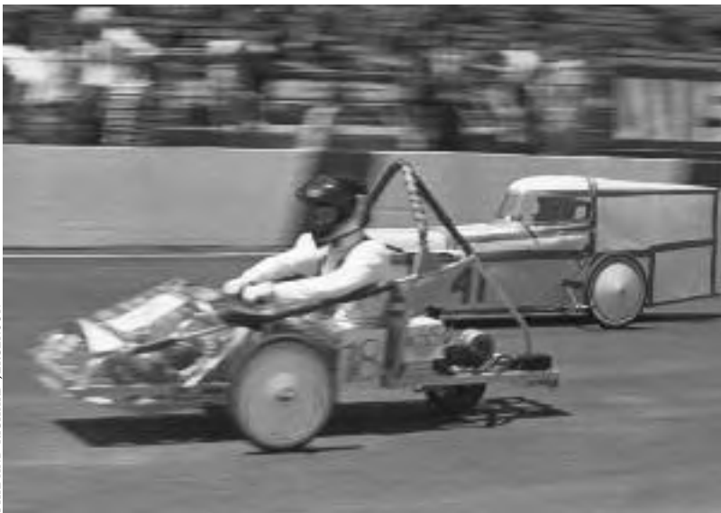
11.18: Electrathon racing at SEER '92. Built by students at Willits High School, the nearer vehicle has a grid beam frame.
