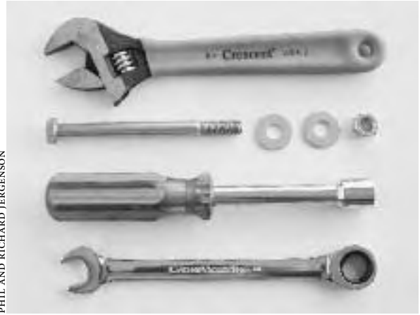
1.8: Basic tools and fasteners for metal-frame projects. The nut driver and gear wrench at the bottom of the picture really speed assembly.
