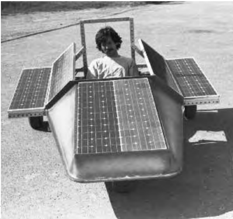
11.14: Phil in the X-Wing, his most fun grid beam vehicle ever. Its low profile — less than 45 inches (1,150 millimeter) including roll bar — kept it stable in high-speed turns.
