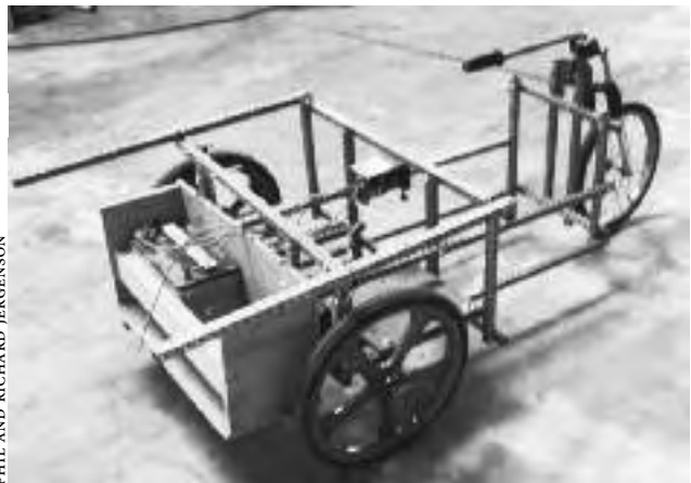
11.6: EVTB trike with wooden battery box.
