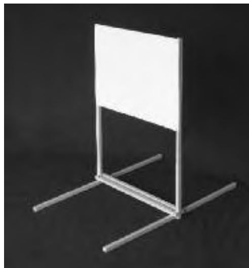
13.19: Model of a 4 x 5 foot roadside sign. Diagonally brace the legs with string or wire.
