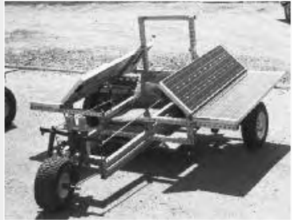
11.15: X-Wing's push rod steering system and home-built leading link front suspension.
