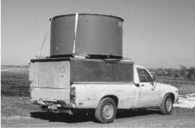
10.2a: Wilma and Tom Blinks built this plywood box around a rack similar to Richard's. Cargo rails on roof, here carrying a 600-pound (270-kilogram) steel tank, were originally supports for a 4 x 7 foot sleeping deck inside.
