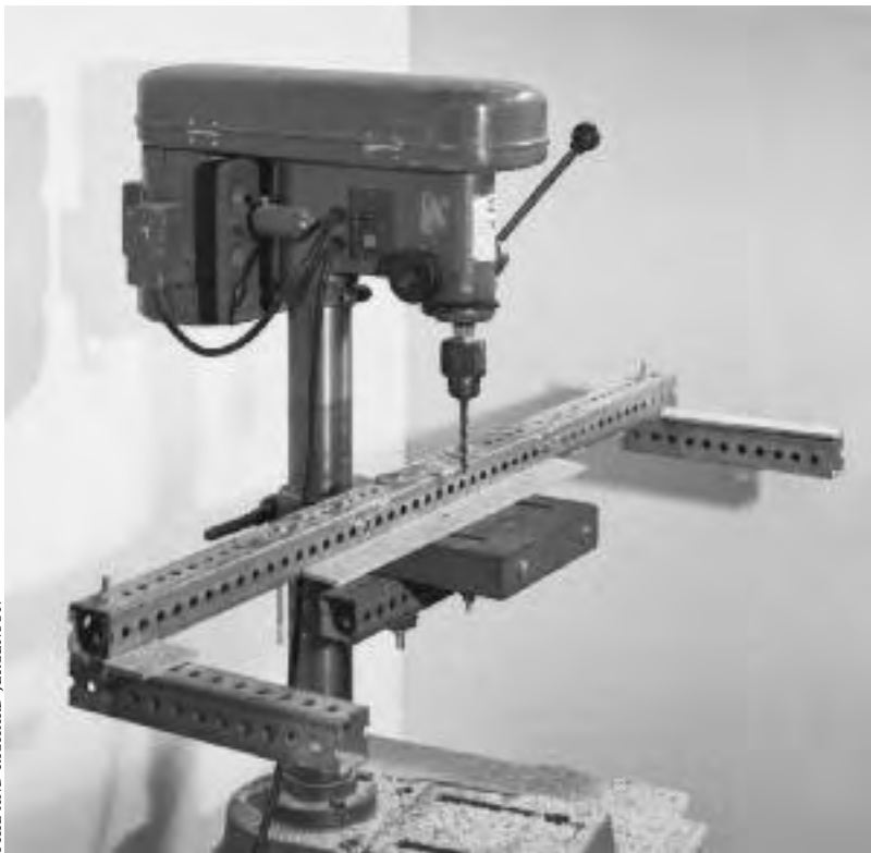
16.6: Drill press with a steel backstop. The support arms keep sticks flat on the table as you drill. To drill wood, add the hardboard backing and spacers shown here.
