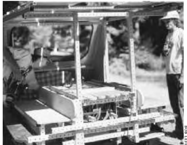
11.26: Richard with the Sol Train on the Fort Bragg to Willits run in 1992. Crossed and stacked frame members create trusses; 1-inch sticks support the solar panel roof.
