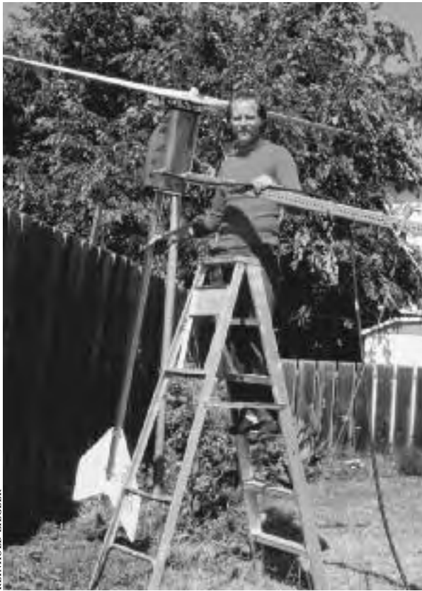
9.6a: Reinhold Ziegler with a student-built wind turbine and tower of 2-inch galvanized steel. Rotor diameter is 7 feet (2,100 mm).
