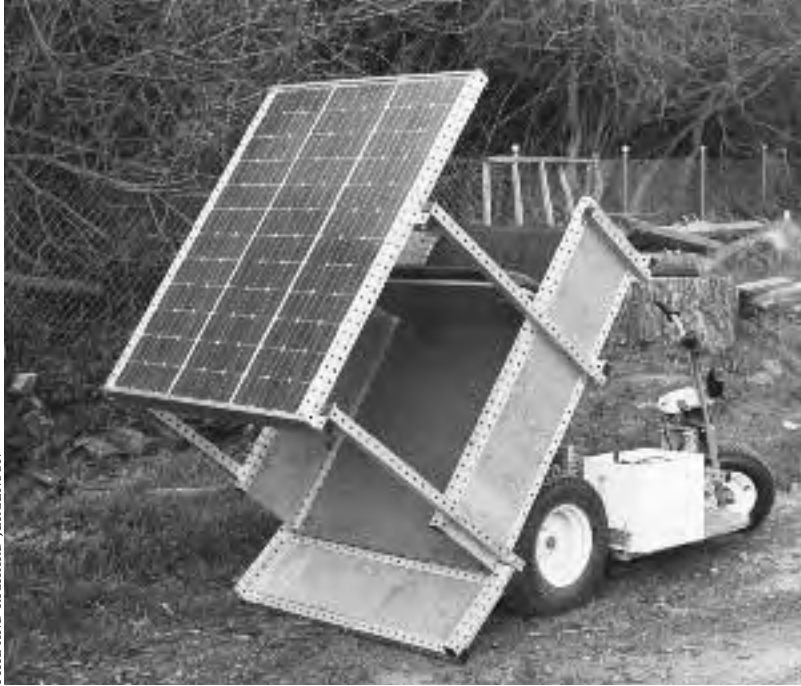
11.11: Tilting the Solar Bear's dump bed aims its solar panels.
