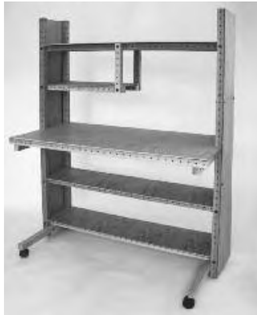
5.5: Phil's computer desk uses shelf and side panels of 1/4-inch plywood. It stands 5 feet high, with a 2 x 4 foot work surface. He later added a back.
