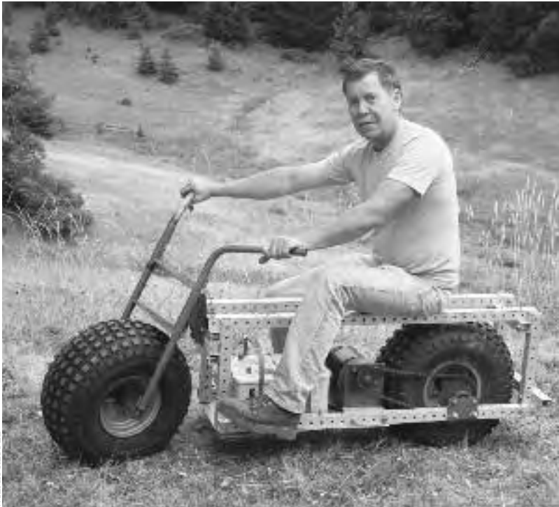
11.9: Phil's Electric Tote Goat demonstrates the simplicity possible with a grid beam frame and drive train. The \frac{3}{4} -horsepower (560-watt) motor is geared directly to the rear wheel.
