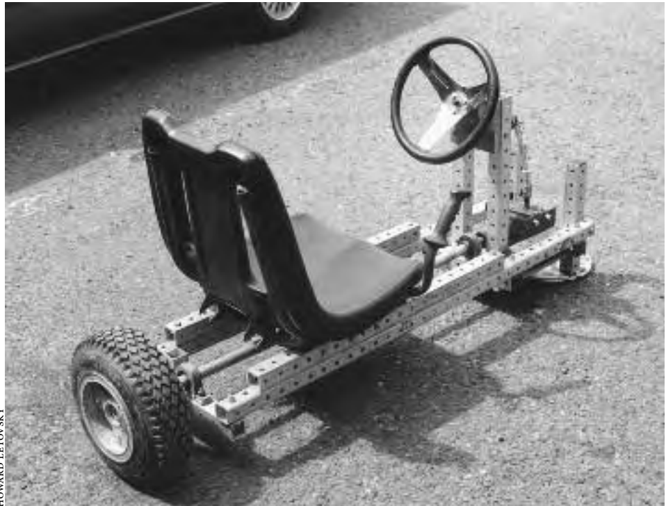
12.3a: Howard Letovsky built this driving simulator prototype in a weekend. The steering wheel rotates the drive wheel in the opposite direction to simulate G-forces.
