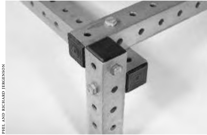
1.6: Tri-joint of aluminum sticks fastened with hex nuts and hex bolts. For a stronger joint, use washers on both sides of the sticks. Press-fit end caps are plastic.
