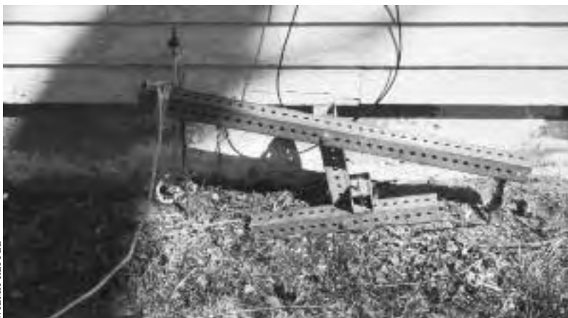
13.14: Wilma's steel-framed lightning rod puller.
