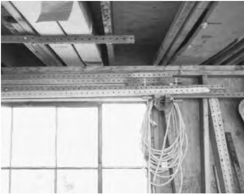
7.12: Grid beam stored overhead between joists, on a rack above a window, and in spaces between wall studs.
