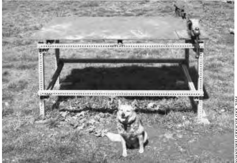
7.4: Kent Jergenson's outdoor workbench has a galvanized steel frame and a plate steel top. As you can see, Kent has many vises.
