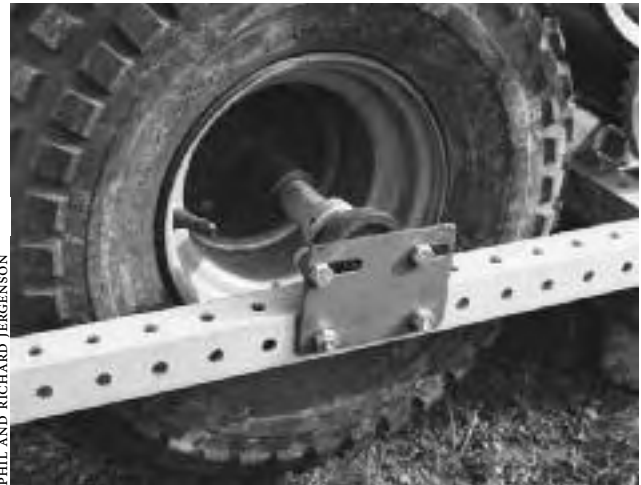
21.7c : Rear wheel mount on Phil's Electric Tote Goat. Slots let Phil adjust wheel position to tension the drive chain.
