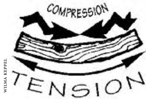
18.10: How a loaded beam bends.
