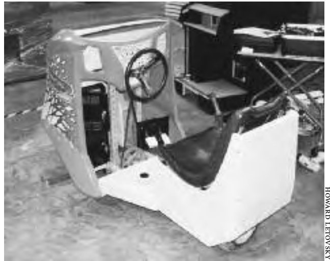
12.3c: This version adds a sturdy front bearing and belt drive, plus an auto seat, plywood rear panels and a plastic front body from a video game.
