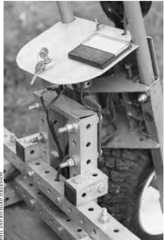
21.11: Solar Bear fork mount, dashboard and headlight. Homemade brake pedal at bottom left pivots on a bolt.
