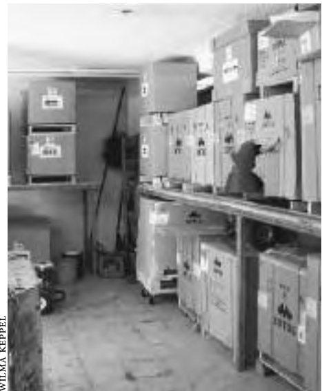
6.4: Steel-framed pallet racks at Earthlab Energy Systems in Willits hold crated wood stoves.
