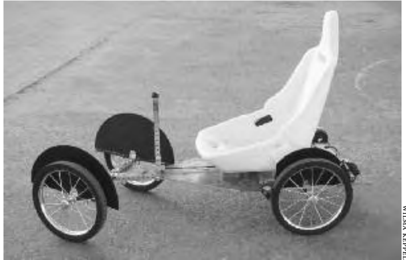
11.21: Eileen Chang's simple go-kart design. The control lever activates throttle and brakes; the driver's feet pivot the bogie-steered front wheels.
