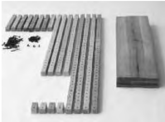
17.4: Bookcase components. All the sticks and panels are standard lengths: 4 sticks 3 inches long; 8 sticks 1 foot long; 4 sticks 5 feet long; 4 sticks 3½ feet long; 4 shelves 3½ feet long
