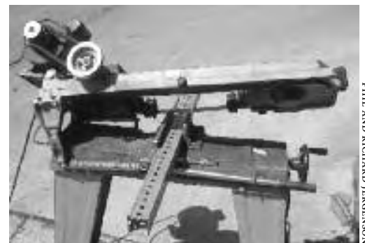
14.4: A band saw is the best tool to cut metal grid beam.
