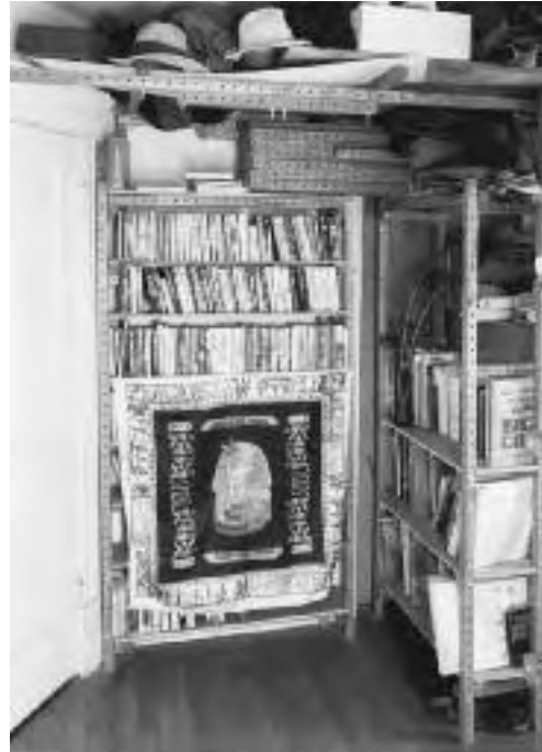
6.5: Shelves for paperback books fit behind door. Bookcases brace each other and support the end of an overhead storage rack holding 400 feet (120 meters) of wooden grid beam.
