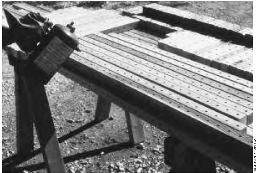
16.12: Applying an oil finish using a spray bottle charged with compressed air. Spray short pieces on top of longer ones so the overspray hits your sticks.
