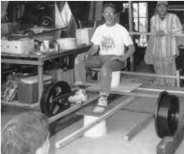
21.3a: Michael Hackleman tests seat position for the Rail Rocket while Kent Jergenson observes. Buckets, wooden sticks and plywood approximate our initial design.
