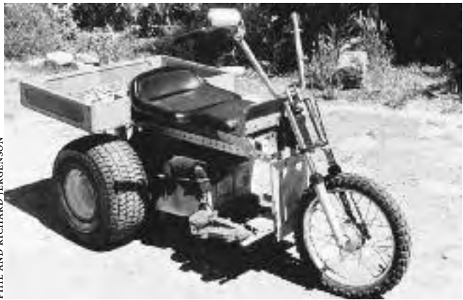
2.8: Phil's 1979 electric Scamp was the first grid beam vehicle framed with aluminum.
