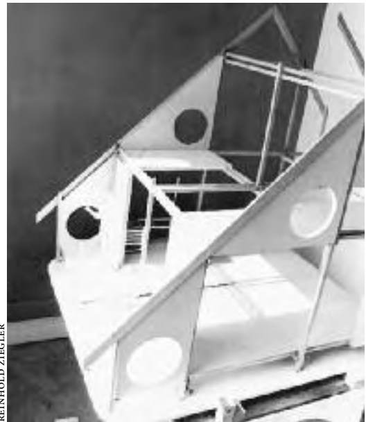
8.16: Model house by Reinhold Ziegler. Sticks are 1/4-inch fir, with cardboard panels.
