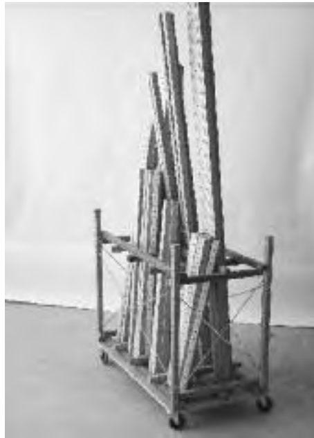
18.6: Tension braces made of threaded rod brace a wood-framed stick rack Wilma built for the Jergensons' shop. Here it holds 300 feet (90 meters) of wooden sticks up to 8 feet long.
