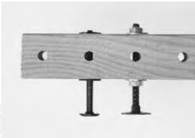
15.7: Leveling feet made with a joint connector bolt and weld nut (left) and an elevator bolt, hex nuts and washers (right).
