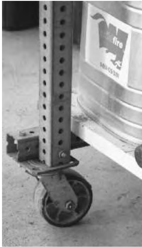
15.5: Holes 4 inches apart bolt an industrial caster to a 2-inch steel workbench frame. Use two or more bolts and support both sides of the mounting plate to keep it from bending.
