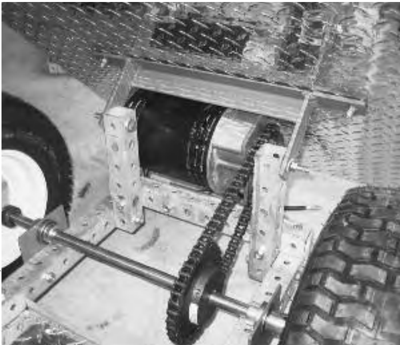
11.2: Simple drive train on a one-speed Yard Truck.
