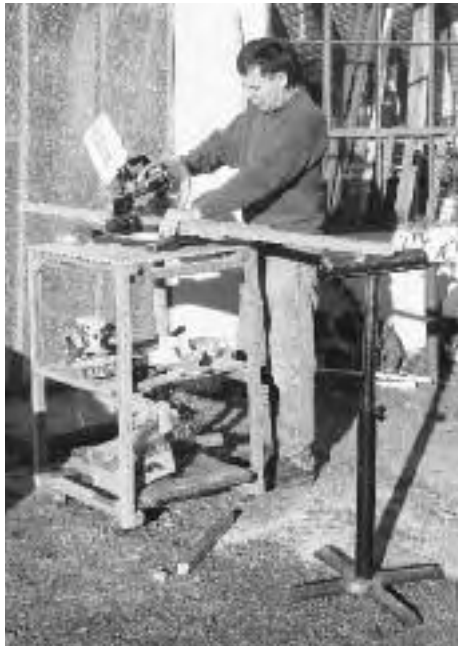
7.5: Wood-framed workbenches are light and easy to move. Phil rolled this one outside to cut sticks using a battery-powered miter saw.
