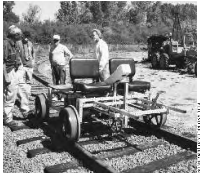
21.3f: Rail Rocket on the track for testing after we removed the pedal drive.
