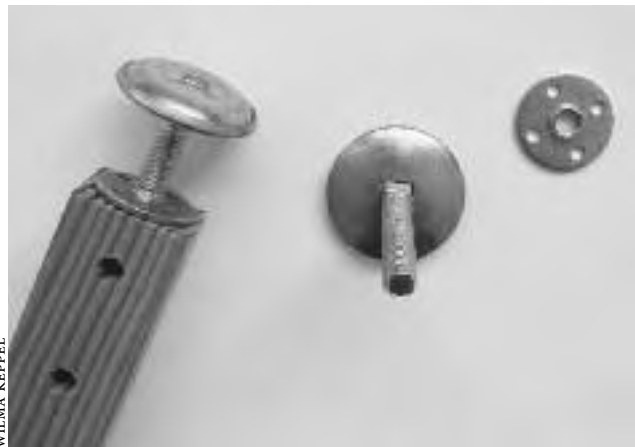
15.8: This screw-adjust foot fits a hole drilled into the end of the stick. Attach the plate with one or more small screws if you wish.
