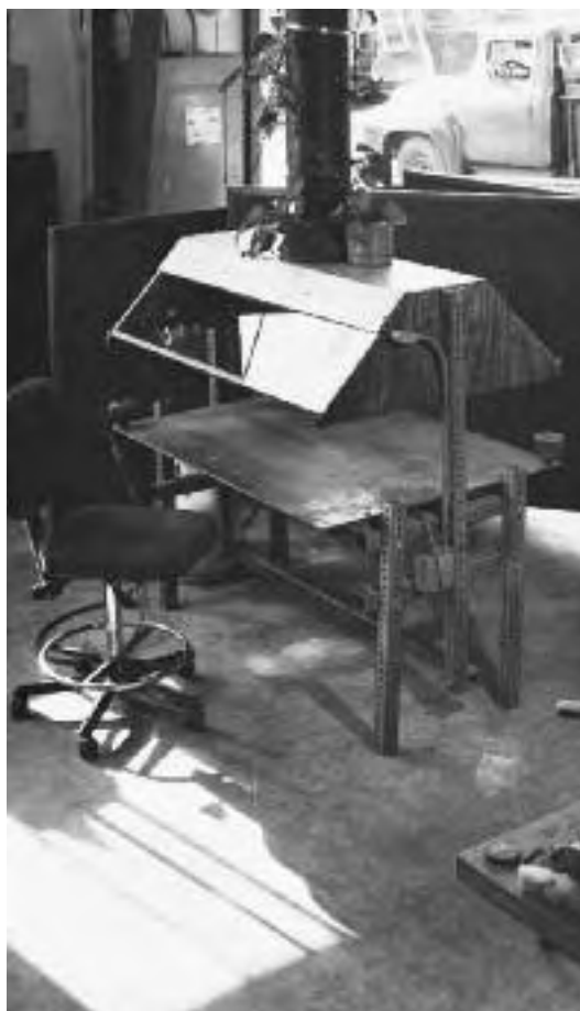
7.1: Soldering bench with vented hood for fumes. Part of a complete industrial assembly line Phil and a colleague built with galvanized steel grid beam in 1980, it's still in use.
